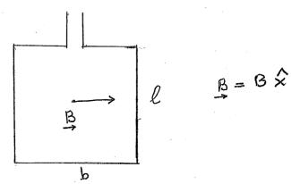
8-14. A coil of cross-section  $\underline{A} = (2 \times 3)m^2\hat{n}$  is being rotated about the vertical in the presence of a constant  $\underline{B} = 0.2Tz$ . What is the maximum and minimum flux of  $\underline{B}$  through the coil? Why?
